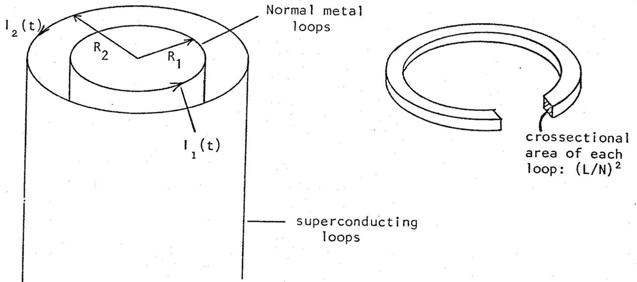
Each solenoid consists of  $N$  identical closed loops, made from wire of square cross-section and of side  $L/N \ll R_1$  or  $R_2$ , as shown.
