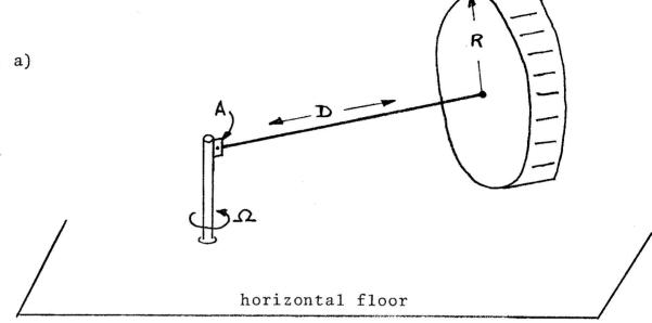
The above figure is a schematic drawing of a mechanism frequently used in mills (for crushing grain) which was known even in Roman times. The horizontal shaft (length D) of the millstone (mass M, radius R) is driven by a vertical shaft. The jointed connection at A enables the millstone to be tilted up or down in the vertical plane. The millstone rolls without slipping on the mill floor.
