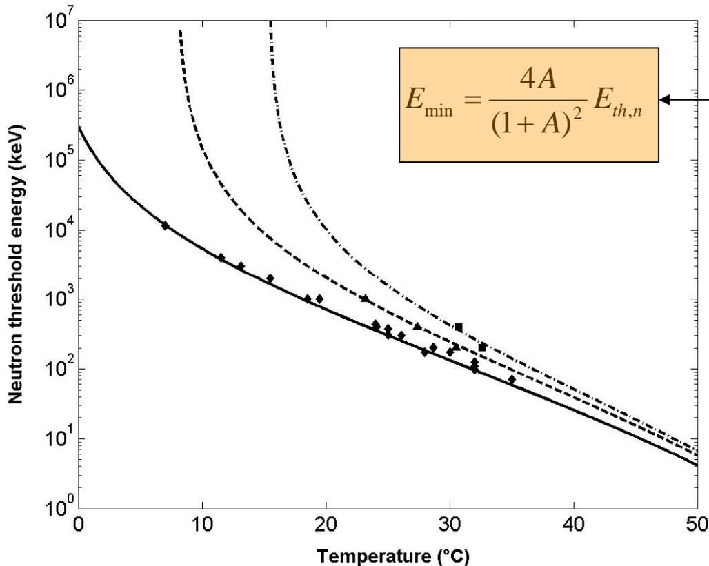
The neutron threshold energy is converted in a minimal energy deposition in the superheated liquid (C<sub>4</sub>F<sub>10</sub>) by considering a maximal nucleus recoil after a neutron-nucleus scattering.
