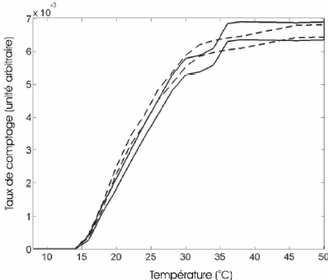
Between 25 and 50°C the alpha response curve shape is unchanged for different droplet distributions. The difference between the curves is due to the smaller alpha response for different droplet mass (geometrical purification)
