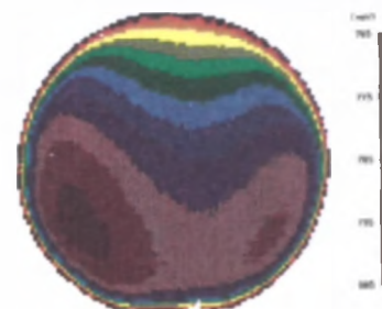
Fig. 3: The peak energy of the photoluminescence emission is mapped for a \text{In}_{0.53}\text{Ga}_{0.47}\text{As} layer deposited by MOCVD. As in Figure 2, the gas flow direction is top to bottom. The InP wafer diameter is 50 mm.
