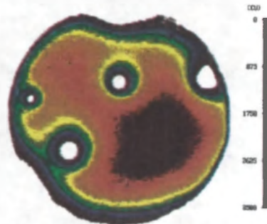
Fig. 5 The photoluminescence intensity at a fixed wavelength is mapped for a MOCVD grown \text{In}_x\text{Ga}_{1-x}\text{As}_y\text{P}_{1-y} layer. The sPL intensity is strongly reduced in the vicinity of particulates which were inadvertently introduced prior to growth. The InP wafer diameter is 50 mm.
