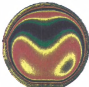
Fig. 2a The reflectance at a wavelength of 1000 nm is displayed for an InP layer grown on an \text{In}_{0.53}\text{Ga}_{0.47}\text{As} marker layer. The red and blue fringes correspond to thicknesses of InP with reflectance extrema at the map wavelength. The InP substrate diameter is 50 mm.
